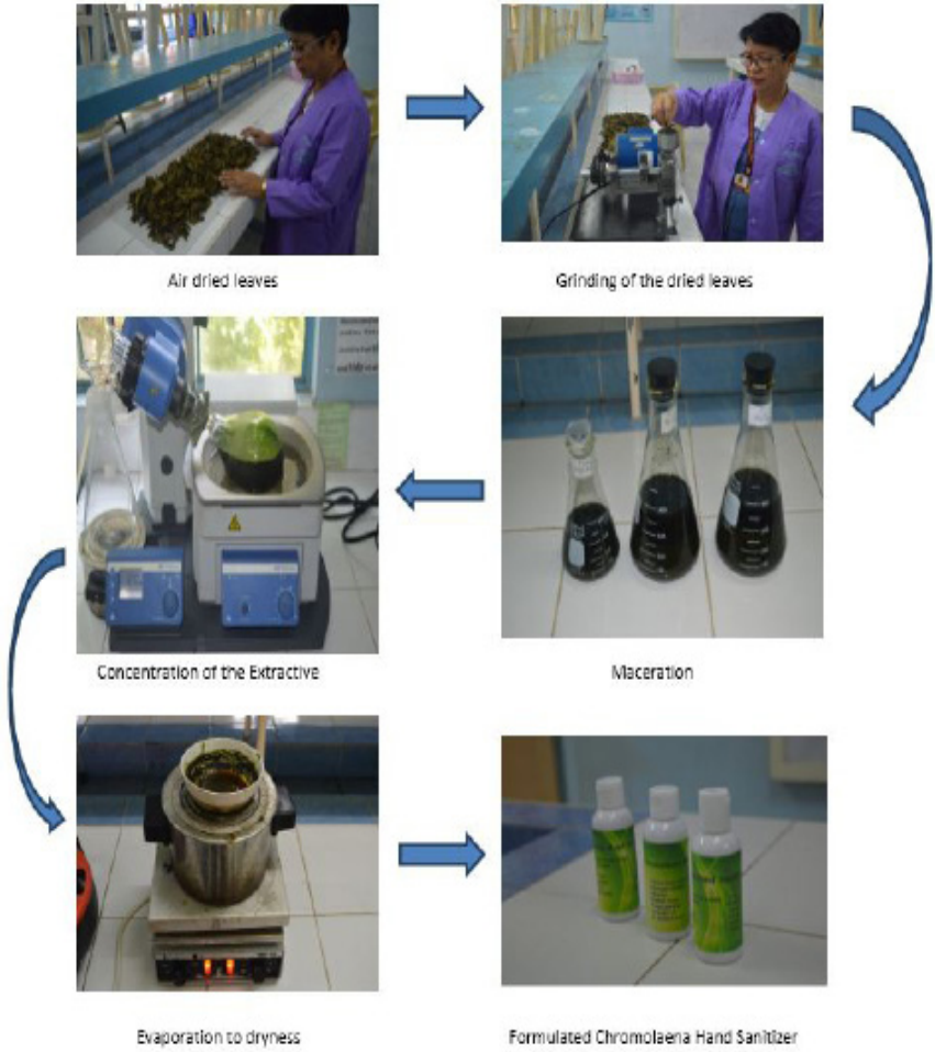
Plate 2. Preparation of Chromolaena odorata leaves extract and formulation of Chromolaena Hand Sanitizer
